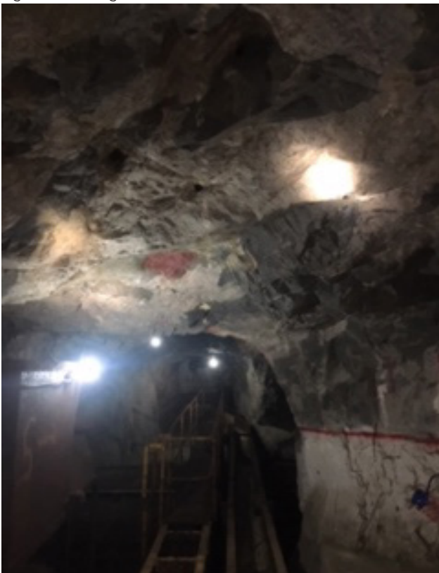
Figure 4: Prieska underground - note no meshing/bolting and good ground conditions
