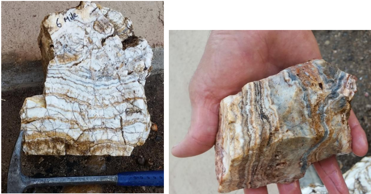
Figure 2: Samples of quartz veins from 6 Mile Creek Prospect demonstrating epithermal textures.
