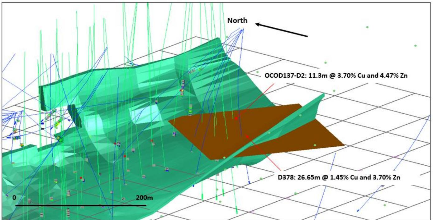
Figure 5: Isometric view of the south-eastern part of the Deep Sulphide Resource (green) showing an off-hole conductive plate (brown) in hole OCOD137\_D2, indicating the continuation of the massive sulphide mineralisation along strike to the south and east.
