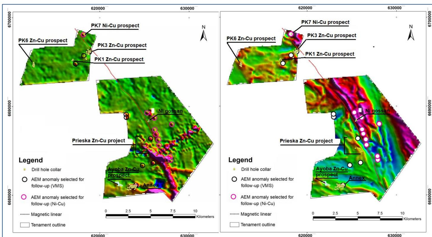
**Figure 2: Airborne EM anomalies shown on the AEM Channel 30 map on the left and on the aeromagnetic map on the right. Hot colours represent high conductivity and high susceptibility. The large, linear conductors south and east of the Prieska Zn-Cu Project are caused by infrastructure.**
